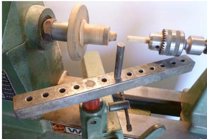
The toolrest used in metal spinning is very different from the kind used in woodturning or machining. Because of the need of a fulcrum for the spinning tool, the toolrest must be able to accommodate toolposts. Throughout the spinning of a piece, the toolposts and toolrest are moved frequently to adjust for the constantly changing outside diameter of the metal.
