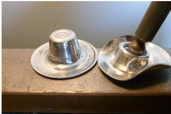
Although not a typical approach in spinning, the Cowboy Hat Pins have several subsequent forming stages not done on the lathe. Knowing that I would dap the top of the hat in, I spun the blank a little taller to account for the metal compressing back down. I used this example to encourage the incorporation of other techniques along with basic metal spinning.
