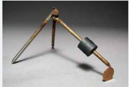
thin "foot" to hold things with minimal heat sink effects and to slip under parts to hold them down
