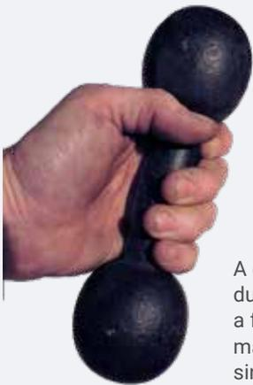
A cast steel dumbbell (\$5 at a flea market) makes a superb sinking hammer for making bowls.
