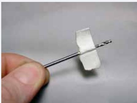
When you need to blow away dust from where you are drilling materials or burring wax, make a little propeller to do so, like this.
