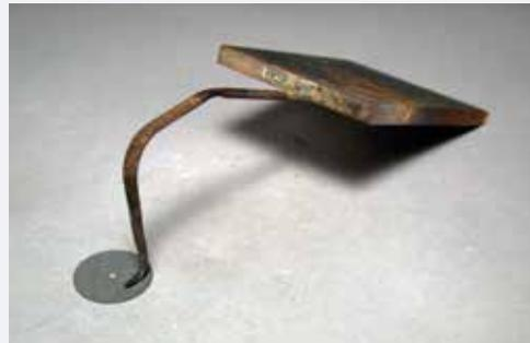
Here is another form of soldering weight that I like; with two of these you can quickly hold most things while soldering. Its weight is increased by stacking a brick or other weight onto the flat surface.
